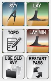
← *LAY MIN (Lay pass with minimum slope)*
